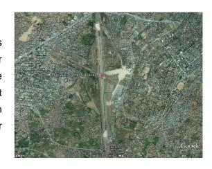
Runway is 2,700m long and 46m wide with 3.0m shoulders on either side corresponding to International Civil Aviation Organization Category 4E. Aprons are combination of flexible and rigid pavements for passenger and cargo. Nose-in parking for 4 wide-bodied aircraft at a time or 3 Airbus and 2 narrow body aircraft at a time is possible.
